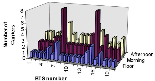
Figure 9: The number of carriers required per macro-cell BTS (for BTSs 1 to 20 of Les Vosges network) for the traffic floor, the morning and the afternoon traffic load distribution.
