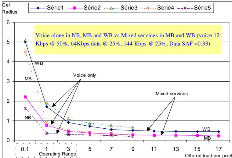
Figure 1. Cell size results from CDMA Initial dimensioning
