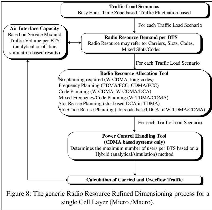
Figure 8: The generic Radio Resource Refined Dimensioning process for a single Cell Layer (Micro /Macro).
