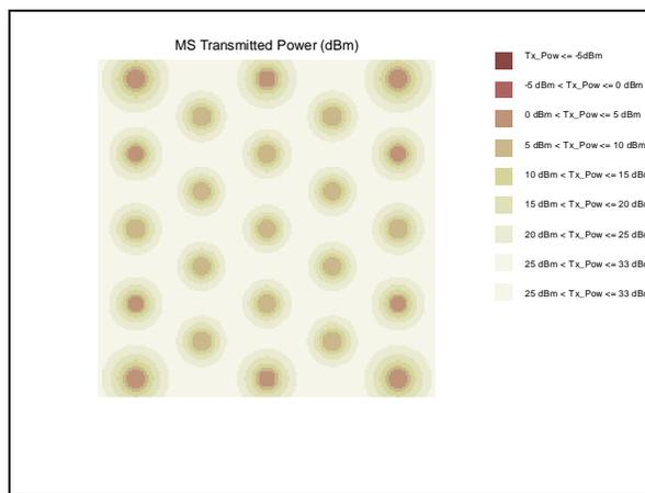
Figure 10: Power Control Tool in CDMA dimensioning: Mobile transmitted power distribution at the final iteration of the process
