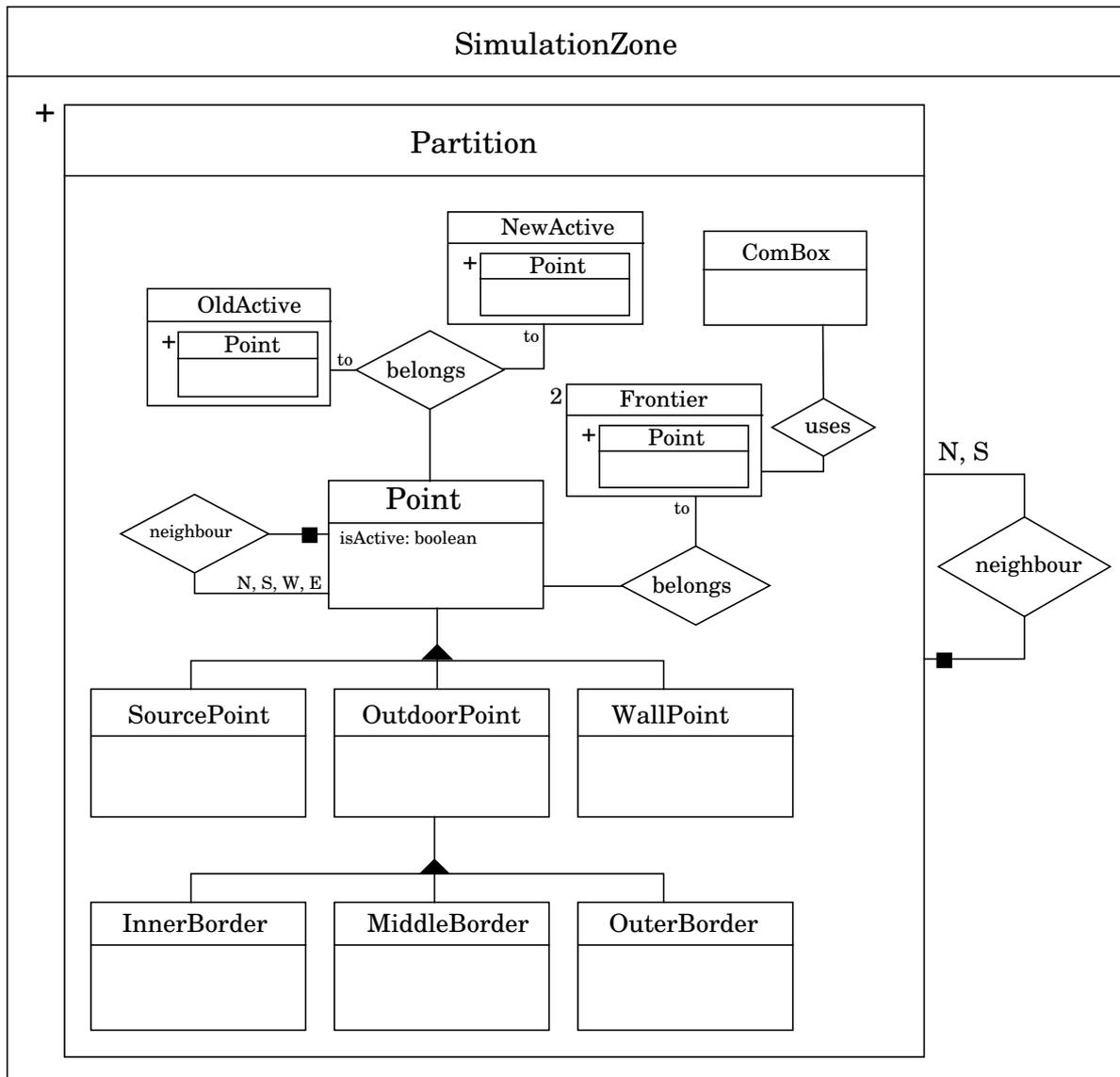
Figure 5: Fusion object model of the ParFlow++ software
