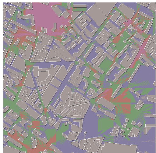
Fig. 13 A solution obtained, with a 160 individual population, after 320 generations. The 36 selected BTSs cover 94.09% of the initially covered surface.
