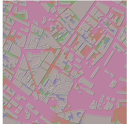
Fig.12 Coverage obtained with the 99 potential BTSs. Pink locations are covered 4 or more times.
